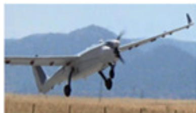
USOL - K150 MTOW: 150 kg Payload: 50 Kg Endurance: 18 HORAS Take-off / Landing: PISTA
