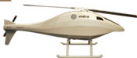
INDRA - PELICANO MTOW: 200 kg Payload: 30 Kg Endurance: 8 HORAS Take-off: Catapulta Landing: Paracaidas
