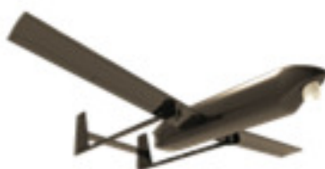
AERTEC - TARSIS 75 MTOW: 75 kg Payload: 12 Kg Endurance: 8 HORAS Take-off: Catapulta Landing: Paracaidas
